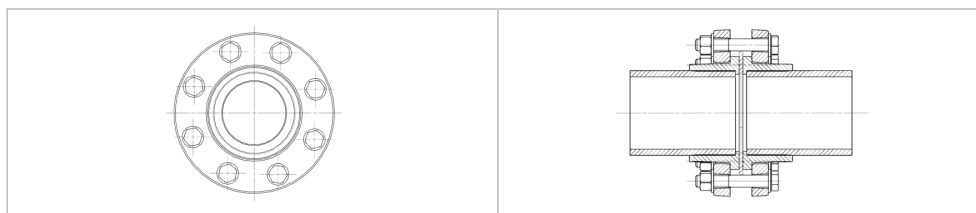
Flange with main axes (centered, crosswise)
