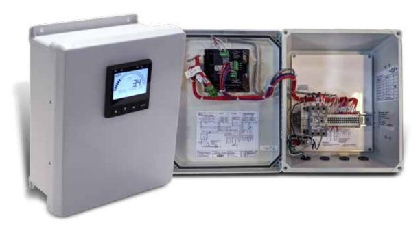
Instrument enclosures offer a simple solution, for the customer, who might not have the time to install and wire transmitters into panels. Whether it's a standard 9900 / 9950 or something more custom, these panels make installation easy. Just mount the instrument enclosure, wire the sensor, and any outputs to the prewired - labeled DIN rail mounted terminals. With the DIN rail mounted 24VDC power supply (equipped with a 6 ft. 120 VAC power cord), the enclosure is a plug and play system.
