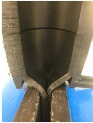
Coupling Crush Test: PASSING
