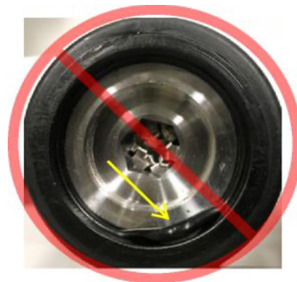
O-ring pinched and displaced
