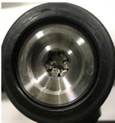
O-ring properly seated against punch
