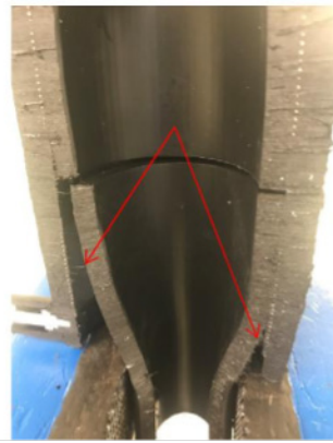
Coupling Crush Test: FAILURE
