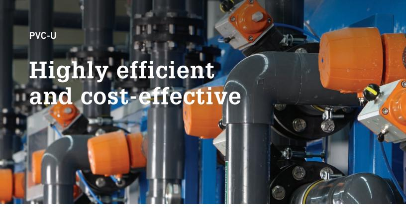
The assortment covers the dimension range from d6 to d400 (metric) and 3/8" to 8" (British Standard), and can be used up to a maximum temperature of 60°C. The maximum system pressure is 16 bar. The guaranteed compatibility between the individual system components simplifies and accelerates assembly, and significantly reduces installation costs.
