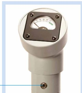
The meter is calibrated 0-100 to indicate a peak response to the Pulse Transmitter signal
