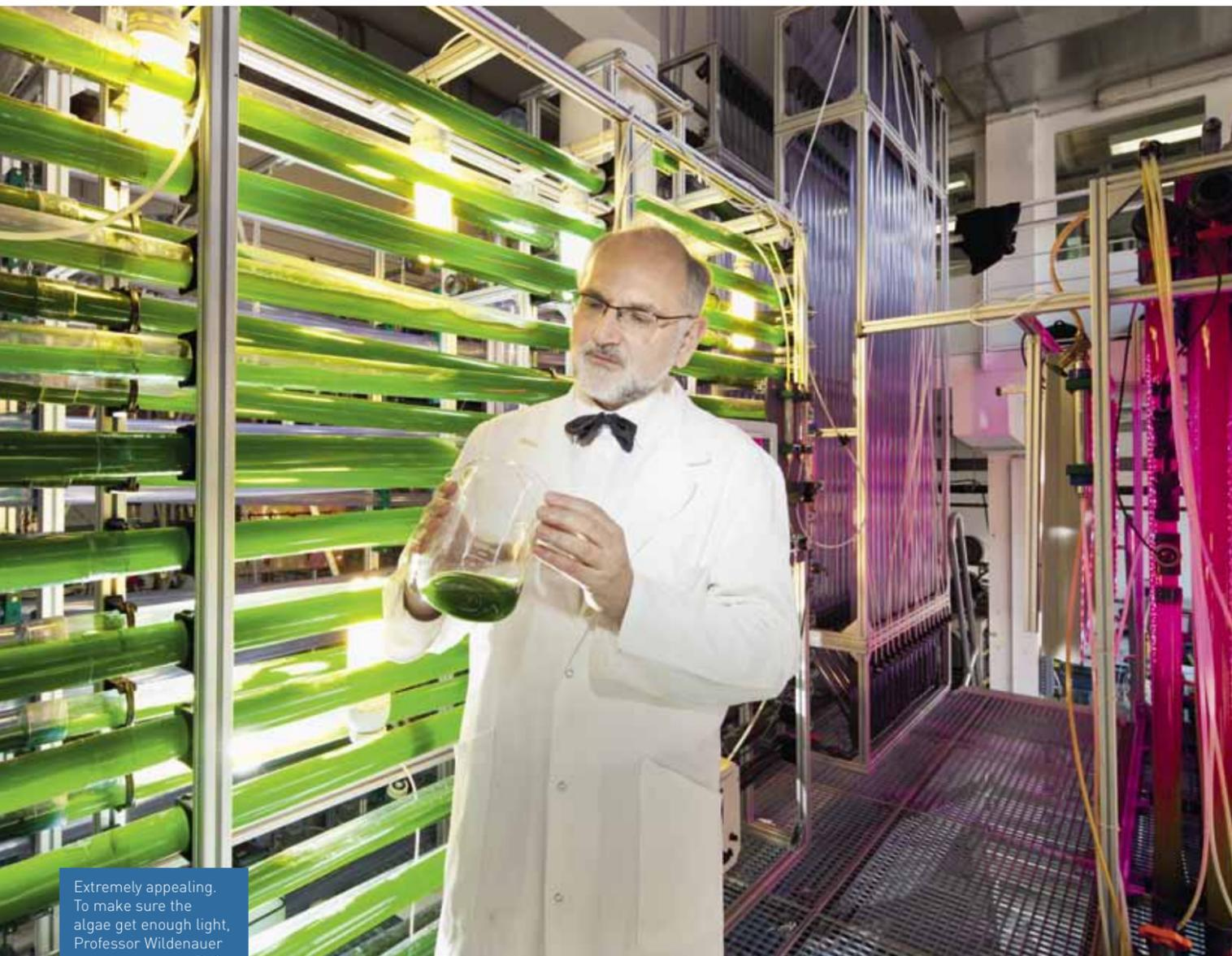
Extremely appealing. To make sure the algae get enough light, Professor Wildenauer uses transparent PVC tubing manufactured by GF Piping Systems.
