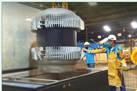
Water Tank (Hydro-Pressure Test 1200mm PE Pipe)
