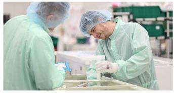
The SYGEF Plus (PVDF-HP) is double-bagged to ensure highest safety and cleanliness standards.
