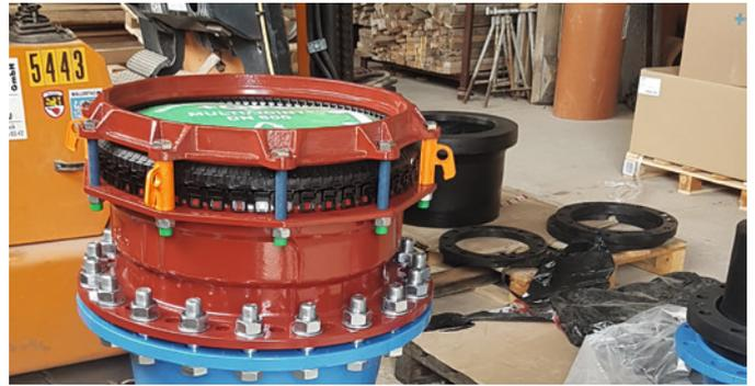
MULTI/JOINT 3000 Plus: Fast and safe material transition, also for DN 500.
