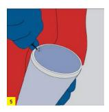
Remove the burrs on the external edges with a knife or scraper.
