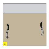
Mark the pipe clamp distances properly with 1% inclination on the wall or ceiling where they will be installed. (as flat wall)
