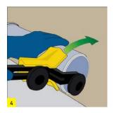
Chamfer the spigot of pipe by using a chamfering device or thick riffler.
