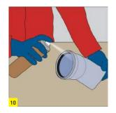
Apply a lubricating liquid (silicone etc.) to the socket part of the pipe.
