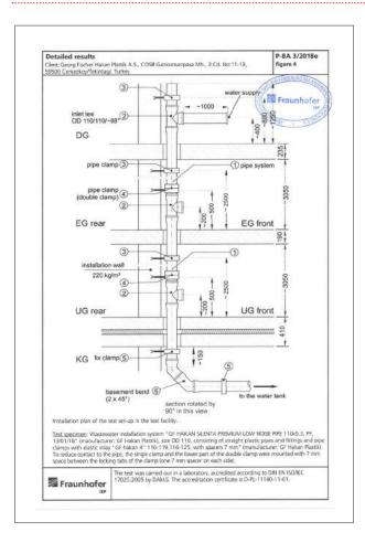
To achieve maximum acoustic performance, the silent pipe clamps used in the test should be used in the installations as well.
