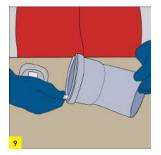
Mark the part of the pipe that will be attached to the fitting as much as the jointing distance.
