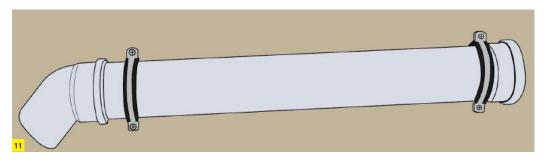
After the pipe and fittings are jointed, place them and tighten the clamps.
