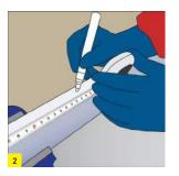
When interval measurements are required, mark the pipe with the desired measurements.
