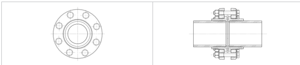
Flange with main axes (centered, crosswise)
