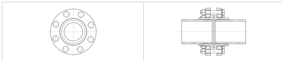
Flange with main axes (centered, crosswise)
