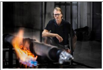
HEAT-FIT Jacket System, composed of pipes, fittings, and valves being fire tested.
