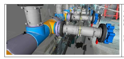
The replacement manifolds were designed by 3D-scanning the existing systems.
