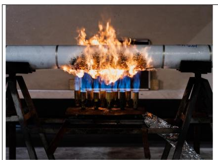
The HEAT-FIT Jacket System was subjected to a variety of fire resistance tests.
