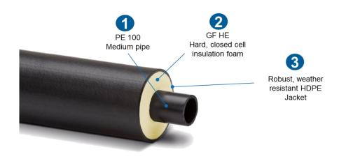
Pre-insulated 3-in-1 layered structure of a COOL-FIT 4.0 pipe
