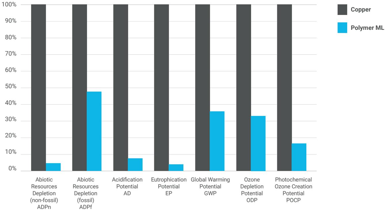
**Environmental profile of the Polymer/Al/Polymer composite pipe system for hot and cold water in the building from cradle-to-grave per functional unit**
