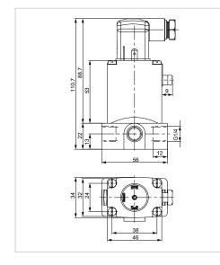
Mounting: By drilling M4 × 8 (metal housing) or self-tapping screws (plastic housing) on underside of the housing on the hole pattern  $38 \times 24$ .
