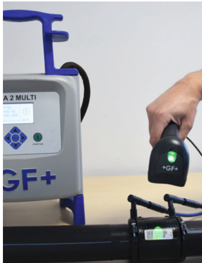
Reliable welding: Quality control protocol and barcode reader card for data input.
