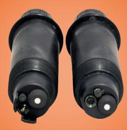
Process electrodes built with superior glass formulation, 3-electrode differential design and protected reference electrode housed in a glass half-cell to withstand extreme pH conditions, elevated temperatures and poisoning ions. These sensors are suitable for continuous monitoring of pH and ORP in a wide range of heavy duty applications.
