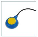
The type 2285 floats on top of the fluid being measured due to its relative density being less than that of water. The level switch is triggered when the internal contact reaches the +/- 45 from horizontal switching angle.
