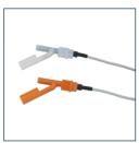
The switch is mounted on the side of the vessel. A hinged plastic float with a magnet floats up and down thrugh the liquid level. The encapsulated reed contact is operated by the magnet.
