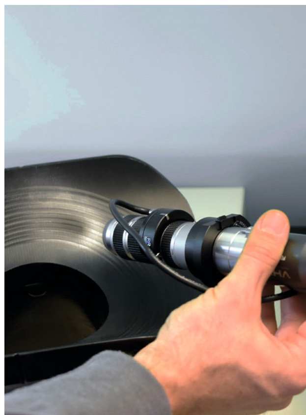
Visual quality control of the welding zone at the ELGEF Plus Branch Saddle Topload
