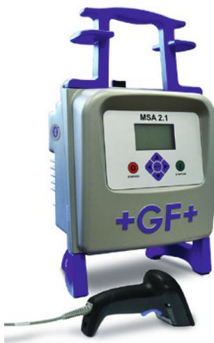
The MSA 2.1 automatic electro fusion unit combines light weight and high efficiency, thanks to its inverter technology and furthermore provides fusion documentation in PDF. The unit is extremely fast and simple, with three basic operations required to operator: connect, scan, start the fusion. It is robust, safe and ergonomic.
