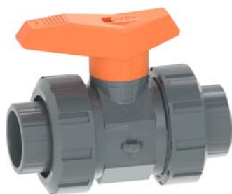
Ball valve type 542 PVC-U With cemented socket (BS) With PTFE ball seal
