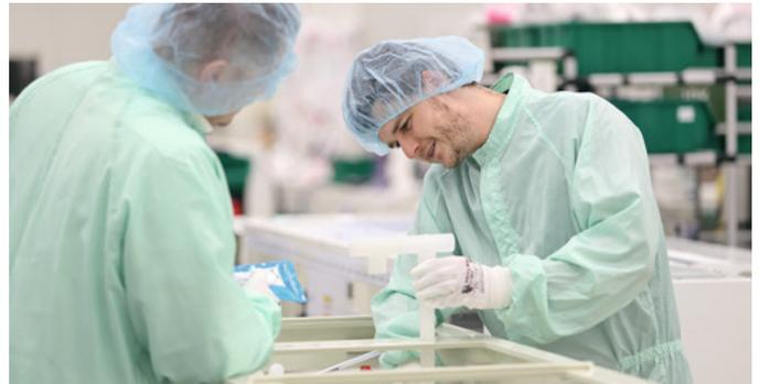
The SYGEF Plus (PVDF-HP) is double-bagged to ensure highest safety and cleanliness standards.
