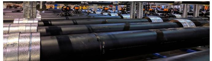
Prefabricated pipe modules ready to be shipped to the construction site.
