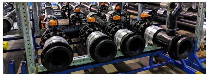
Prefabricated pipe modules ready to be shipped to the construction site.
