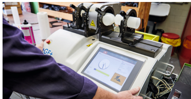
Automated IR welding technology ensures maximum safety and reliability.
