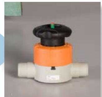
**12** Attach the handwheel to the spindle. Don't apply pressure, just turn it slightly until it falls onto the spindle. There should be a "click". For final testing, open the valve completely and see whether the housing nut is still tight.
