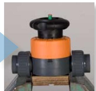
**12** Attach the handwheel to the spindle. Don't apply force, just turn it slightly until it falls onto the spindle. There should be a "click". For final testing, open the valve completely and see whether the housing nut is still tight.
