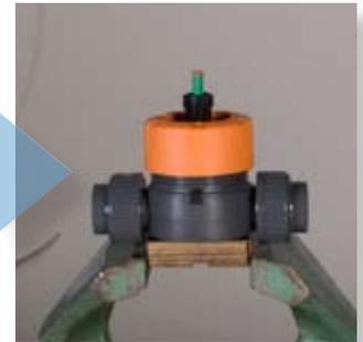
**8** Hand tighten the housing nut as far as you can.
