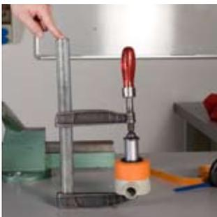
**9** Use a C-clamp to pre-tension the inner housing. Tighten the housing nut to the dedicated position
