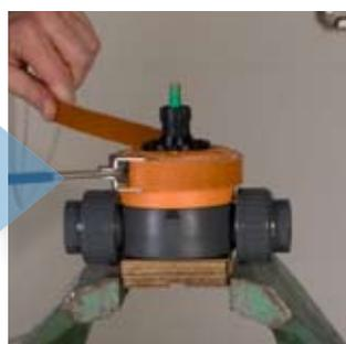
**10** ...to tighten the housing nut, till...
