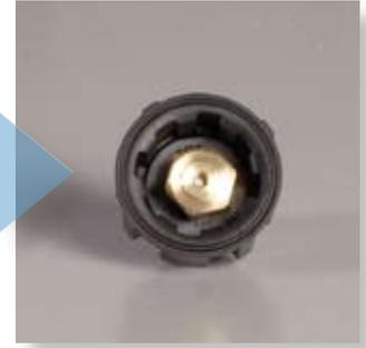
**4** Check if the spindle assembly sits proper in the inner housing. Attach the compressor, if it is poised proper, there is no need to press it in.
